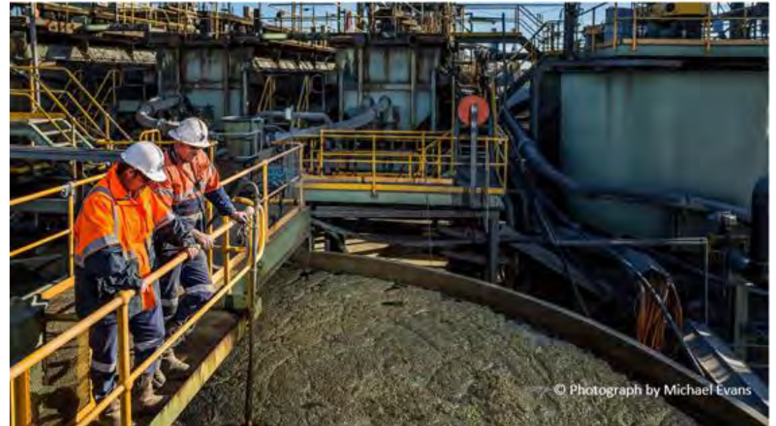
Use of flow rate meter to measure slurry of cement, tailings, and water
