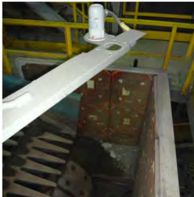
Fig. 4: The controller regulates conveyor speed based on the ore level signal from the ABB LM80 laser level gauge
